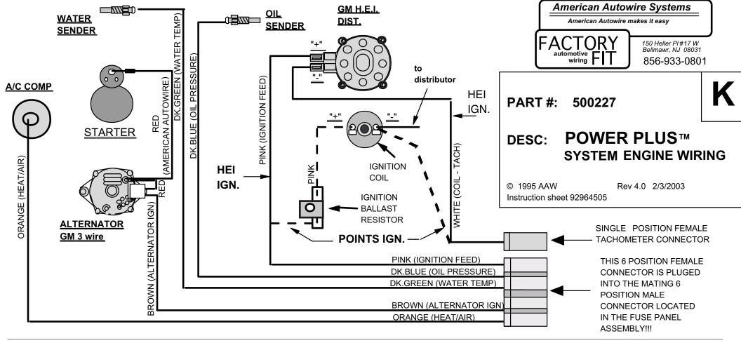
We recommend connecting the engine harness to the mating connector in the fuse panel harness first and then routing the wiring into the engine compartment. By laying out the wiring in this manner, you will be able to select the best points to make your cuts for the individual component connections. Completion of the engine harness wiring will then proceed as follows:
